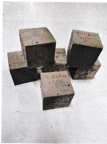
Figure 6: Mortar cubes for the strength index test: Figures from left to right indicates GP control, mortar with 650°C calcined clay and mortar with 800°C calcined clay respectively
