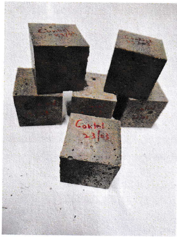
Figure 6: Mortar cubes for the strength index test: Figures from left to right indicates GP control, mortar with 650°C calcined clay and mortar with 800°C calcined clay respectively
